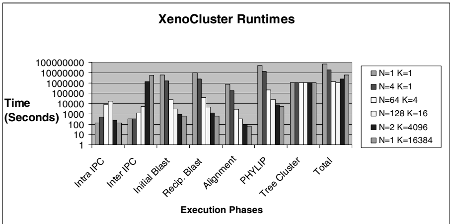
Fig. 5. XenoCluster execution times for varying number of clusters and cluster sizes. Total number of compute nodes varies from 1 to 16384
