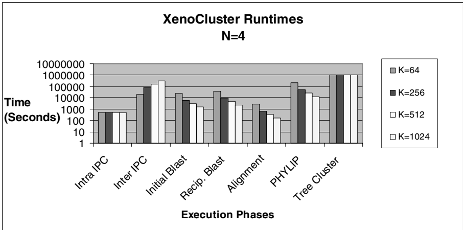
Fig. 4. XenoCluster component execution times with cluster size (N) fixed, number of clusters (K) varying. Number of compute nodes varies from 256 to 4096
