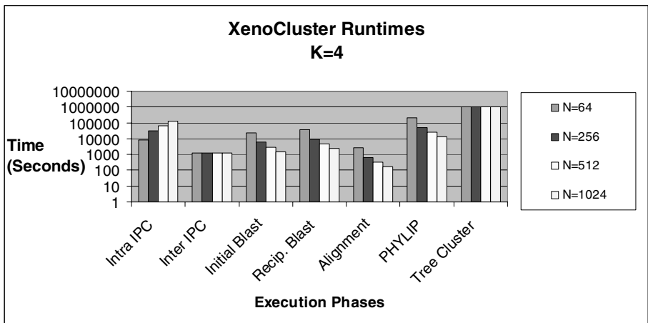
Fig. 3. XenoCluster component execution times with number of clusters ( K ) fixed, cluster size ( N ) varying. Total number of compute nodes varies from 256 to 4096
